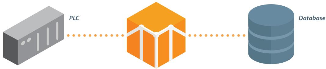
*The SQL Bridge Module allows two-way communication between a database and your PLC.*
